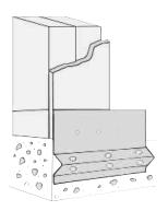
Refer to ASTM C1063 for support spacing, lath selection, fastener selection and further information regarding the proper installation of metal lath.
