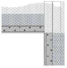
Refer to ASTM C1063 for support spacing, lath selection, fastener selection and further information regarding the proper installation of metal lath.
