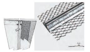
**Zinc Control Joint** has a solid flange with large holes that aid in the attachment of adjoining metal lath. The improved shoulder design allows for easier stucco embedment and increases holding capacity at the joint to minimize cracking. CJ comes pre-taped to ensure a clean joint. Produced in 10' lengths.
