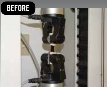
Initial sample of ARMORFLEX placed in Instron Testing Equipment.
