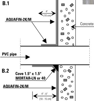
**AQUAFIN SEALING GASKET:**Size: 18" x18" (450 x 450 mm) can be cut to required size and shape
