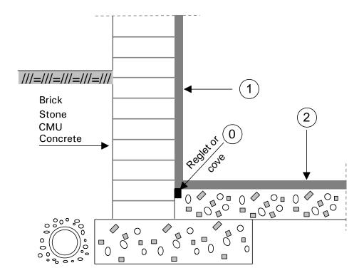
O Install sealing reglet (~1" x 3/4") or cove (~1.5" x 1.5") with AQUAFIN-MORTAR-LN at wall/slab joints.
