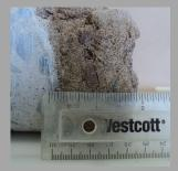
InjectPro-PM3811 Series of acrylates penetrate deep into soils to solidify the substrate and adjustable curing times allow for better control over depth of penetration.
