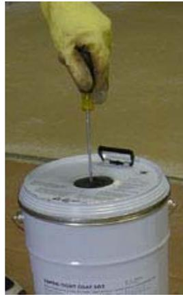
2. Pierce a hole through the top (rubber membrane) and the bottom of Part B.
