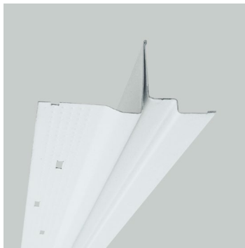
Shadow Reveal Transition Molding 9/16" Shadow Reveal Transition Molding; 120", 3/8 x 1/4" shadow reveal with 9/16" horizontal flange • 7911
