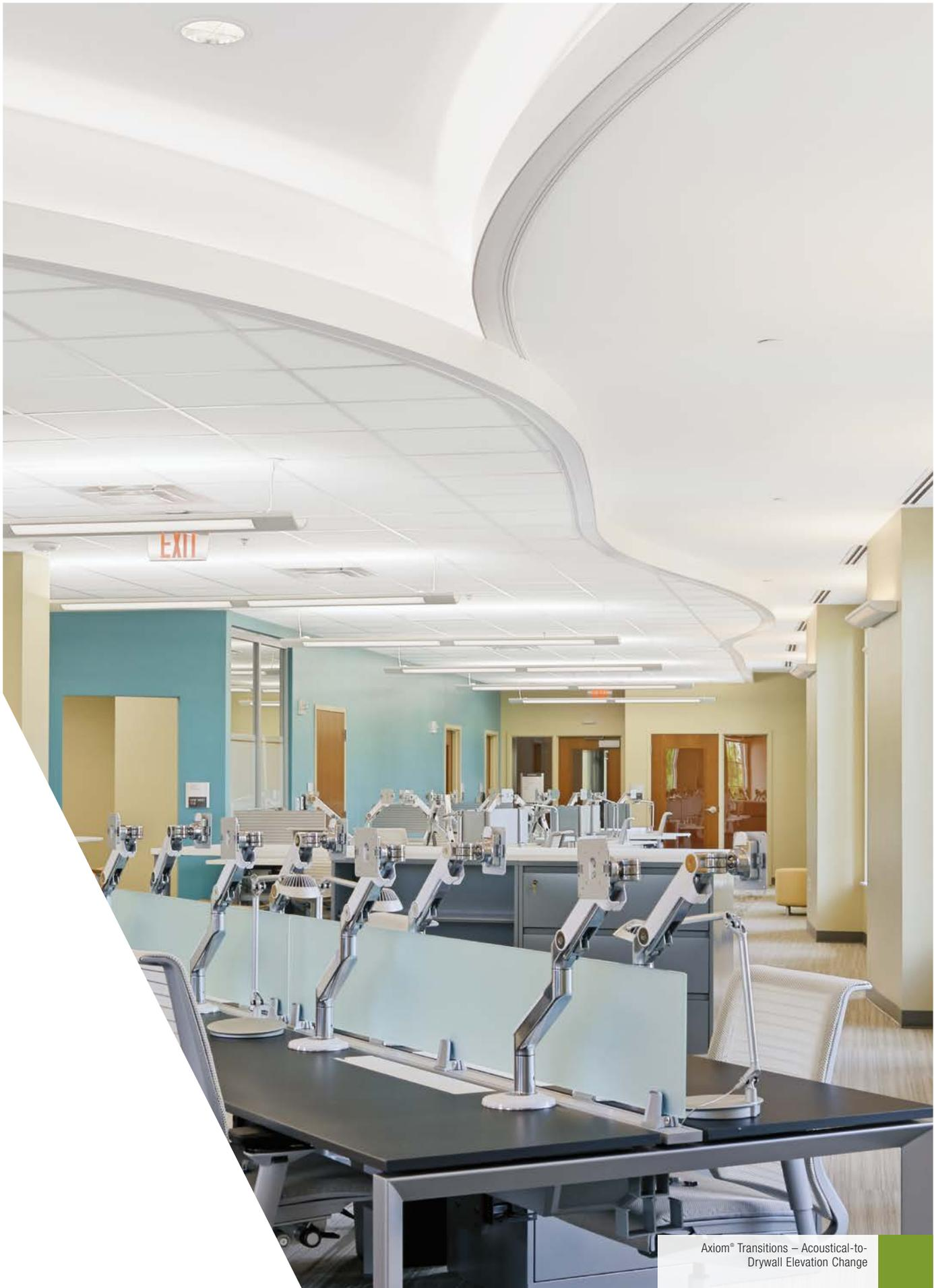
Axiom® Transitions – Acoustical-to-Drywall Elevation Change
