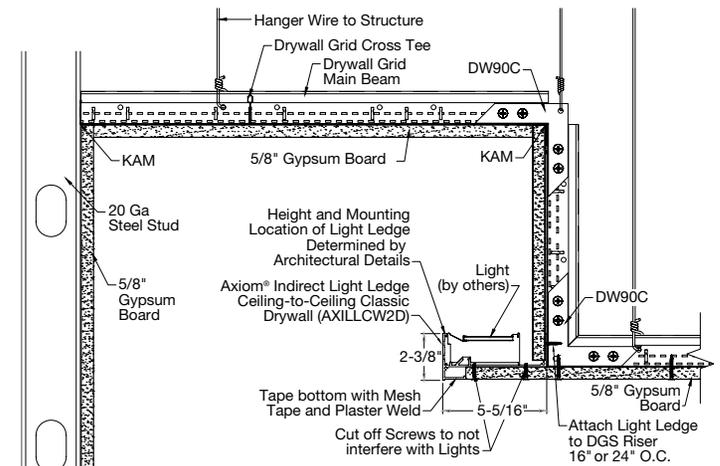
Axiom® Indirect Light Ledge Corners can be ordered in both the Knife Edge® trim and 2" Classic drywall trim for both Ceiling-to-Wall and the Ceiling-to-Ceiling conditions. The pre-made, factory-finished inside and outside corners are made to match the trim option of the straight or curved Axiom trim sections. Each corner section is 12" by 12" square (dimension taken on the face of the extrusion) **(Fig 4) (Fig 5)**.
