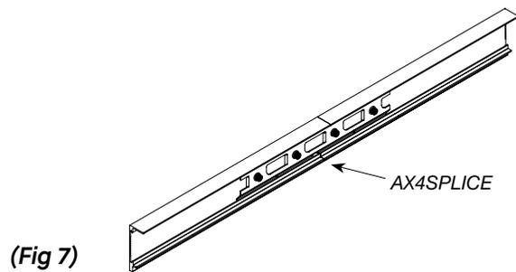
**NOTE:** Splice plates can slide completely into the channel bosses and then slide into the adjoining section after the ledge is aligned. This will aid splice plate connections for the last piece.
