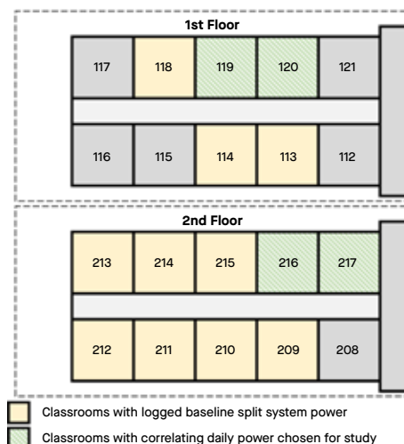
Figure 1b: Classroom wing showing monitored rooms
