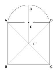
**Step 5:** Using point E as the center point, and dimension E - Aas the radius, form the primary vault from points A to D.
