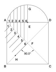
**Step 9:** Transfer length of each line created in Step 7 to corresponding lines created in Step 8. This will create curve points of the groin vault.
