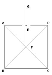
**Step 4:** Layout line F - G beginning at point F, running through point E, equal in length to side A - B. Point G represents the top of the vault, and line F - G represents the centerline of the vault.
