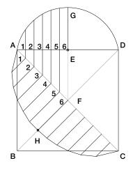
**Step 11:** Form the groin vault by connecting the points created in Steps 9 and 10.
