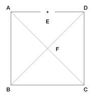
**Step 3:** Layout diagonal lines A - C and B - D - these are the groin lines. Label the intersection of these lines F.
