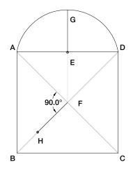
**Step 6:** Use the rise of the primary vault (E - G) and locate the rise of the groin vault (F - H).
