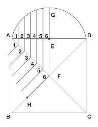
**Step 8:** Mark and run lines perpendicular to line A - C at each of the points created in Step 7.
