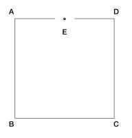
**Step 2:** Determine the midpoint of line A - D and label E. This is the radius point for the primary vaults.
