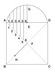
**Step 7:** Run lines parallel to line F - G at one foot intervals beginning at point E and moving towards point A. Number the points where these lines intersect the diagonal (A - C) beginning at point A.
