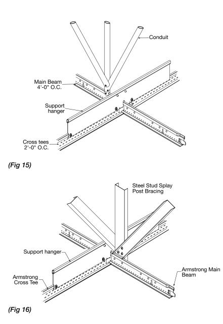
**9.2.5** Rigid bracing at all four corners meets the requirements of Seismic Design Categories D, E, and F for clouds up to 200 SF as long as:
