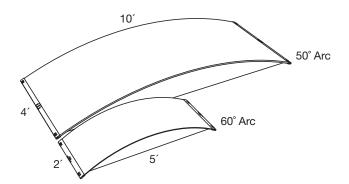
The elevations would be different with these two different size canopies linked side-by-side.
