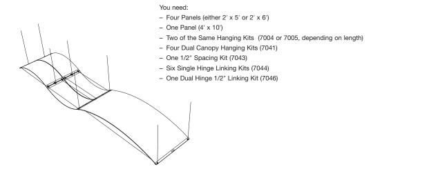
To Create: Four Small Canopies and Two Large Canopies in This Configuration
