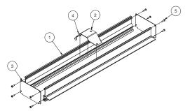
If drywall is already installed, take care to mark fixture openings on the face of the drywall for future rotozipping of the fixture opening. The fixture kit can then be installed from above and the fixture can be screwed in to the drywall grid flange. NOTE: Use 1-1/4" (6#) self-tapping screws when screwing kit flange into drywall grid flange. In this instance, the drywall will be penetrated with a screw. Over-tightening of the screw can cause the drywall to crack.
