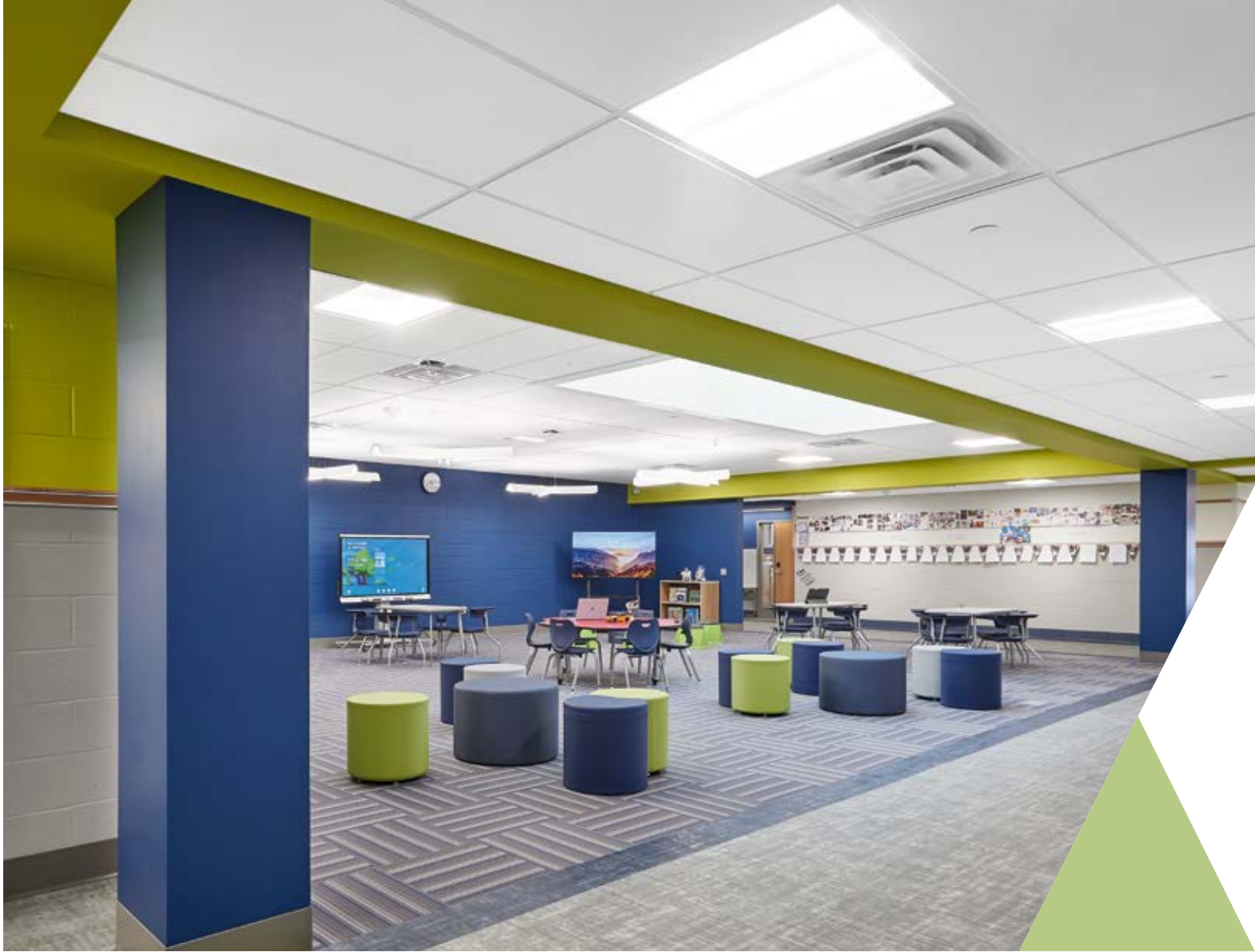
▲ Ultima® Ceiling Panels with Prelude® 15/16" Suspension Systems; Loganville Elementary School, Loganville PA; RLPS Architects
