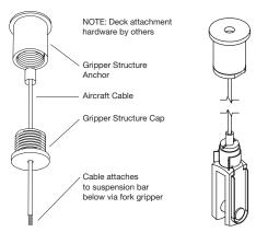
**NOTE:** In cases where attachment to structure is not possible at 24" centers, hanging kit assemblies can be spaced at a maximum of 36" O.C. along the length of the bar and within 12" of each end of the bar. (holes for the Attachment Pin will have to be drilled in the field).
