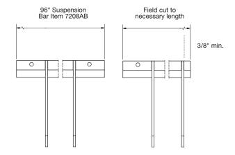
To touch up cut ends of the suspension bar, use a commercially available matte black paint.
