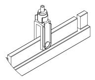
8. Runs of suspension bars can be achieved using the end-to-end connector (item 6651AB).
