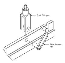
7. Slip the attachment pin through the fork and hole in the suspension system and secure attachment pin to the top of the fork gripper.
