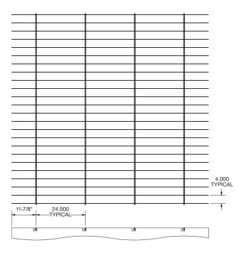
Layouts of suspension bar longer than 8' will require multiple suspension bars to be spliced together. End-to-end connectors (item 6651AB) are required to splice the suspension bars together and maintain proper spacing and alignment.
