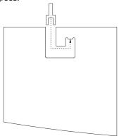
Each blade is attached to the suspension system by means of hanging the factory hook cut out in the blade over the vertical flange of the suspension bar.
