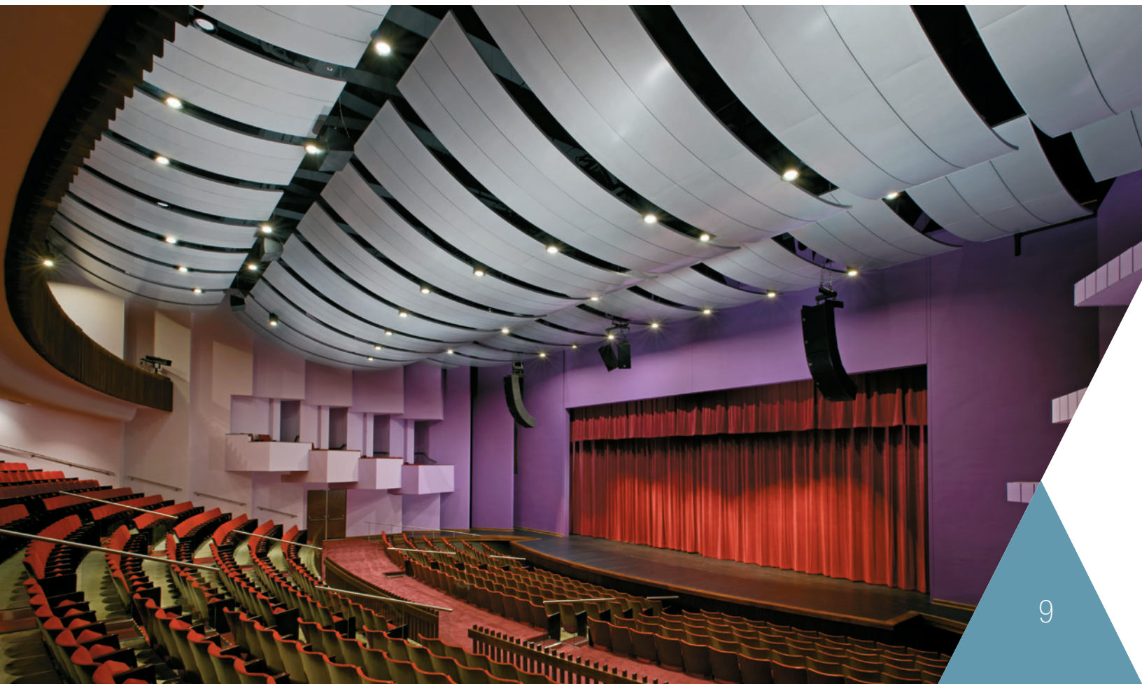
▼ Serpentina® Waves™ Acoustical Clouds 2' x 8', 2' x 10' and 2' x 12' panels with R062 perforation in Silver Satin; Lewis & Clark Community College, Godfrey, IL
