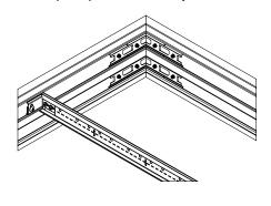
To secure splice plates for straight trim joints, pull the trim tightly together for the best fit. Use a 1/8" hex key wrench to tighten the set screws that secure splice to trim. CAUTION: Do not over-tighten these screws to the point where they distort the face of the trim.
