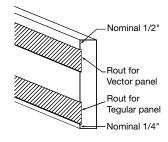
For full sized Woodworks Tegular panels using 9/16" grid, cut a miter on each end of each side of the trim so the measurement from long point to long point is 1 15/16" larger than the nominal dimension of the cloud.
