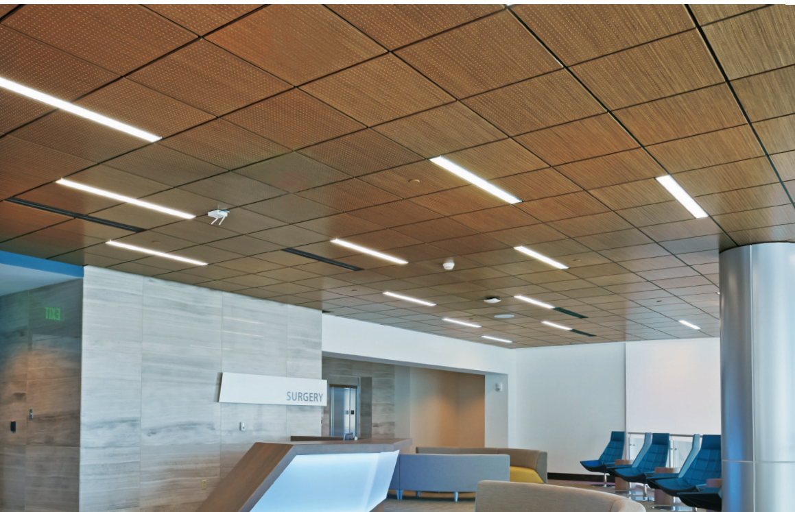
▲ WoodWorks® Tegular panels with W2 perforation in Natural Variations™ Maple with Suprafine® XL® 9/16" exposed tee suspension system
