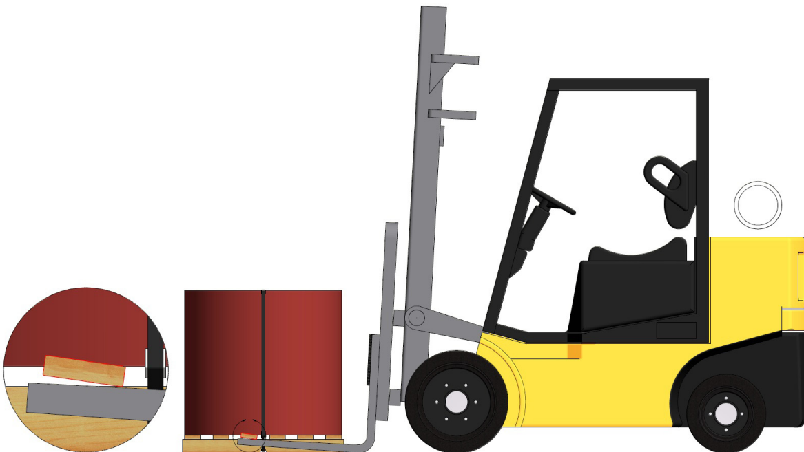
Figure B5. When forks are too short to support the entire skid, the tips may break cross members and damage the coil sidewall.
