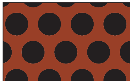
A25 3/8" holes | 9/16" staggered centers 40% open area | Shown in Mission Red
