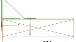
(A) Install 24 GA Cant with 3" Leveling Angle onto Substrate and Roof Membrane.
