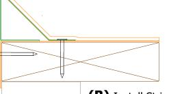
**(B)** Install Strip-in Membrane over top of 24 GA Cant per Membrane Manufacturer's Directions.
