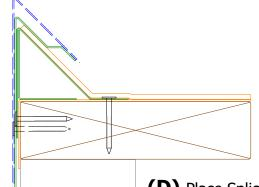
**(D)** Place Splice Plates at ends of Inside/Outside Miters and at the ends of the Straight Fascia Covers.
