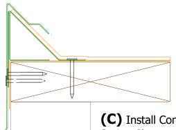
**(C)** Install Continuous Spring Cleat on top of Strip-in Membrane and 24 GA Cant.
