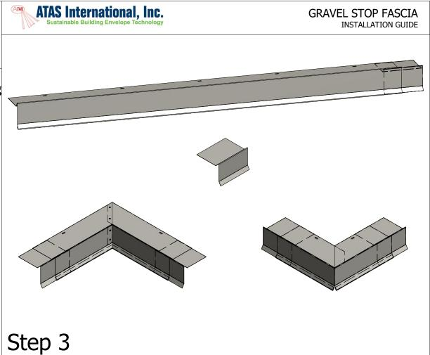
4) Install Gravel Stop miters first. Hook the hem of the Gravel Stop over the cleat and rotate it back onto the roof, taking care to engage both miter legs on the cleat. Secure miter through the roof flange with provided 1 ½" ring shank nails. Install one nail through each slotted hole.
