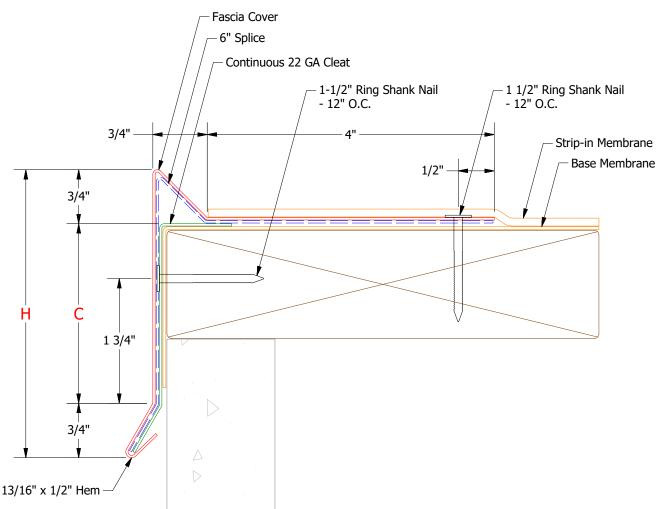
1) Wood blocking must be flush with the face of the wall below. Roof membrane must cover the wood extending 1" below the bottom of the blocking.
