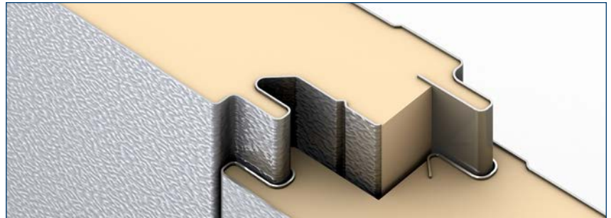
All Isoleren Wall Panels (Isoleren IM, Isoleren ML, Isoleren SL, Isoleren TE, and Isoleren WL) feature the interlock shown above.
