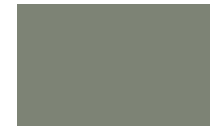
PATINA GREEN Low gloss: SR:0.38 E:0.87 SRI: 41 Std gloss: SR:0.46 E:0.85 SRI: 51
