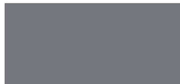
WEATHERED GALVALUME SR: 0.30 E: 0.79 SRI: 27
