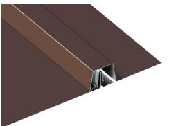
panel, a clip is hooked over the "leg" of the panel, and this is concealed by the batten of the consecutive panel to allow for expansion and contraction. Minimum slope is 2:12 for roof applications. Installation details or hands-on training via seminars are available through ATAS. Visit www.atas.com for more information.
