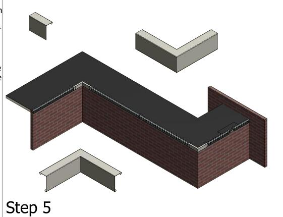
6) Locate covers for end closures, end terms, and scuppers for appropriate locations and positon a splice in the end. Install covers by hooking at top and pressing down to snap into place (see page 4).
