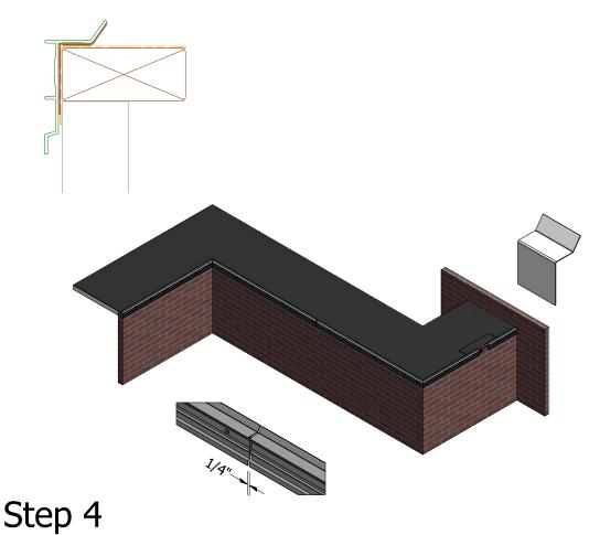
5) Locate miter covers for the appropriate corners and position a splice in each sideof the cover. Hook the top flange of the cover over the top flange of the retainer rotating the cover towards the outside of the building. Press down on the top of the cover to snap the bottom hook onto the bottom of the retainer. Make sure the cover is fully engaged on the retainer (see page 4).
