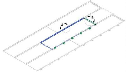
Four way interlock design guards against wind-driven rain and wind uplift, while still allowing for air permeability.
