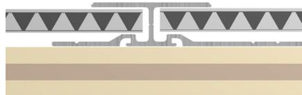
1-Piece, Tight-Fit Flush H Extrusion
