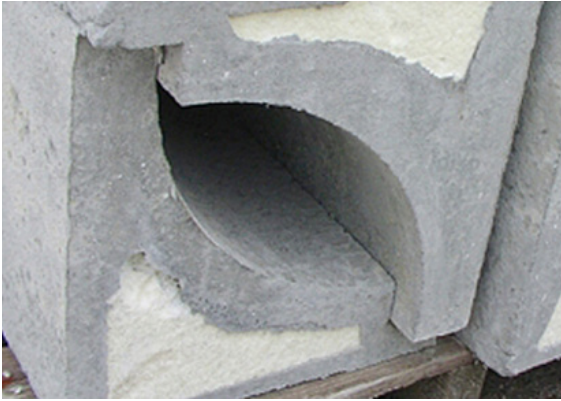
Shown above are pre-cast cornices that have been lightened by using EPS to reduce cost and simplify installation.
