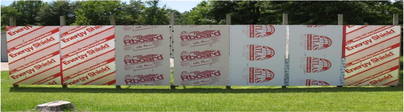
*Fig 2. Mississippi Exposure Test Wall – Courtesy Atlas Wall CI Board division*
