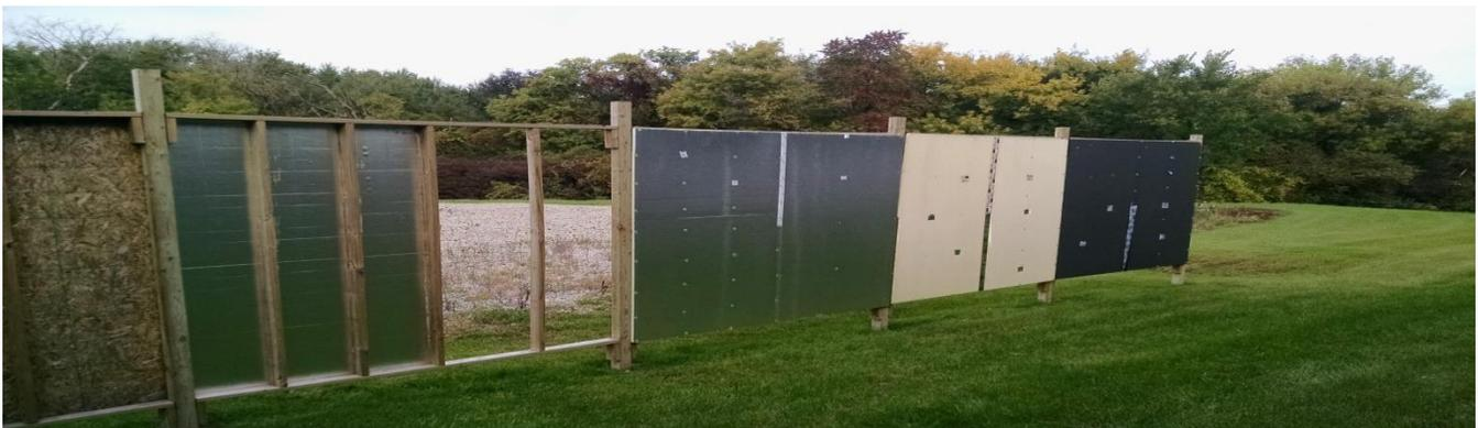
*Fig 1. Michigan Exposure Test Wall – Atlas EPS*
