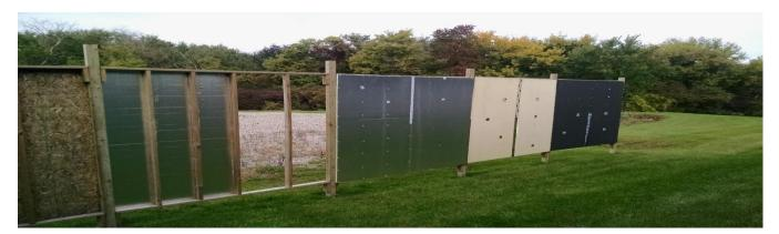
Fig 1. Michigan Exposure Test Wall – Atlas EPS
