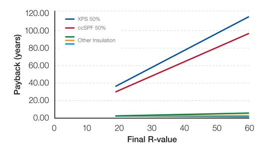
As the thickness of each insulation increases, the R-value also increases. Note that the payback period for EPS, shown in yellow, has a very minimal payback period, even at higher R-values.
