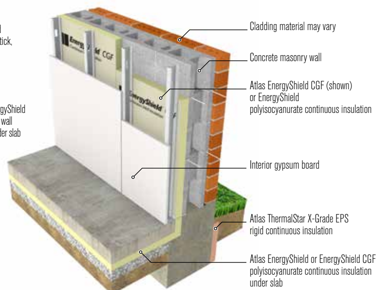
IMAGE 4: MASONRY CAVITY WALL WITH INTERIOR CONTINUOUS INSULATION
