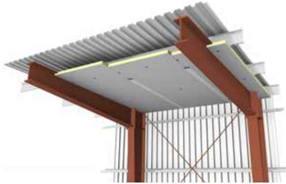
Engineered Metal: Ceiling
