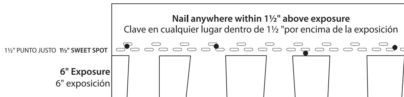
**Note: 6-nail application acceptable where code required; see back for diagram and details**
