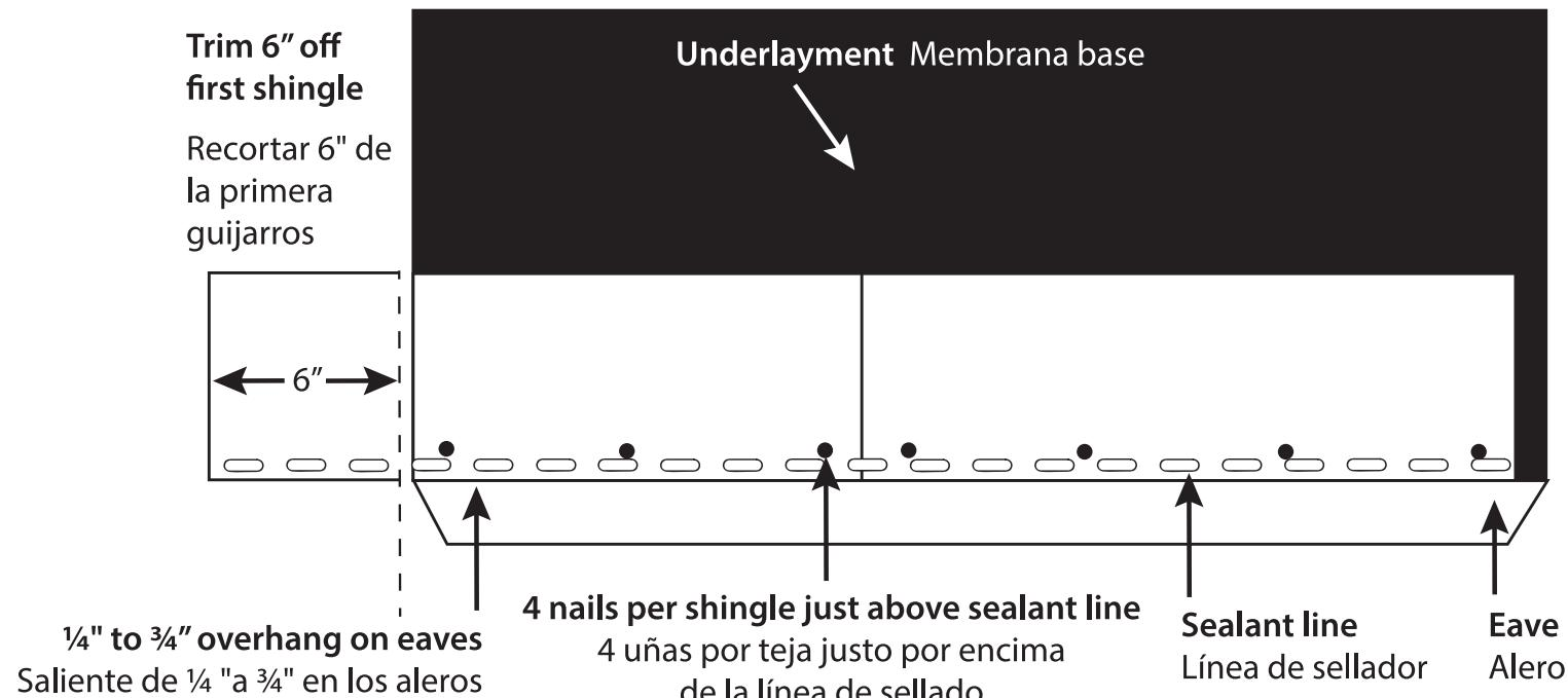
Note: Sealant line should always be positioned facing up at eave
