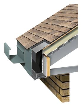
The above image shows the components of the Techni-Flo® EV. Proper installation is required to achieve optimal airflow through the eave and to maintain warranty coverage. Go to www.atlasroofing.com for further installation instructions.
