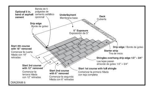
Fourth Course: Cut 18" off a shingle and apply the right half over the third course, flush with the left rake edge, exposing 5". Proceed with full shingles across the roof, maintaining 5" exposure on the course below.
