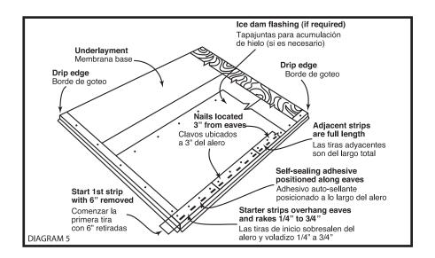
First Course: Begin first full shingle at lower left rake of roof or right of vertical chalk line and continue course across roof with full shingles laid flush with starter course and fastened with 4 nails placed as specified. Note: An optional band of asphalt plastic cement meeting ASTM D-4586 may be applied to the rake of the roof with each shingle course to enhance wind resistance and to resist wind driven rain. See Diagram #6.
