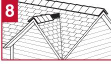
Ridge-to-roof application requires a mitre-cut to maintain continuous ridge line appearance.
