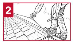
Snap chalk line on both sides of the ridge and no more than .750 (3/4) of an inch from the peak. **Note:** If a ridgepole is present, cut a wider gap to allow a minimum of 1/2" air gap on both sides of the pole into the attic space - but do not remove more than 2-1/4" of roof sheathing material from either side of the ridge.
