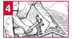
For appearance (to blend with the roof line), it is recommended that the **TruRidge®** vent be installed the entire length of the ridge. Position the first piece at one end of the ridge. Using 2-1/2" nails, for 3/4" deck penetration or penetration through the deck, which ever is less, anchor vent through preformed nail holes.
