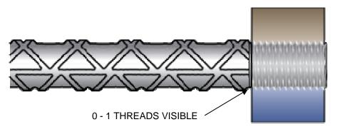
If the threaded rebar end does not properly engage into the Barsplicer DoughNUT Head during assembly, stop immediately. Disassemble to determine the problem. Possible causes of mis-assembly may be either mis-matched thread sizes, or threads are contaminated with (ex.) concrete, dirt, or threads have been damaged. Reassemble only after the problem has been identified and corrected.
