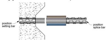
Just before assembly, check both internal and external threads for cleanliness. Clean off any foreign matter. DO NOT USE CORROSIVE ACIDS. Any thread damage must be corrected as noted above before installation.
