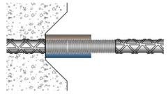
If the threaded rebar end does not properly engage into the Barsplicer coupler during assembly, stop immediately. Disassemble the connection to determine the problem. Possible causes of mis-assembly may be either mis-matched thread sizes, or threads are contaminated with (ex.) concrete, dirt, or threads have been damaged. Reassemble only after the problem has been identified and corrected.
