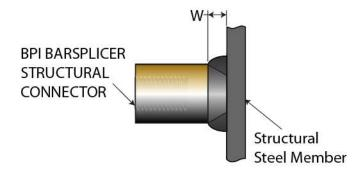
2 When joining the threaded rebar and Barsplicer Structural Connector, remove the protective caps from the bar ends and line up the threaded bar as straight as possible as shown in the pre-assembled condition below.
