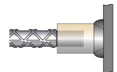
If the threaded rebar end does not properly engage into the Barsplicer Structural Connector during assembly, stop immediately. Disassemble the connection to determine the problem. Possible causes of mis-assembly may be either mis-matched thread sizes, or bars are rubbing against each other, or threads are contaminated with (ex.) concrete, dirt, or threads have been damaged. Reassemble only after the problem has been identified and corrected.
