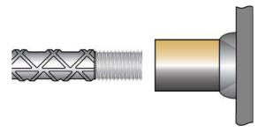
Just before assembly, check both internal and external threads for cleanliness. Clean off any foreign matter. DO NOT USE CORROSIVE ACIDS. Any thread damage must be corrected as noted above before installation.
