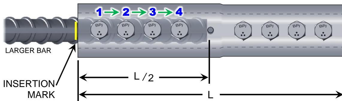
FIGURE 3: **Correct** Tightening Order, 1<sup>ST</sup> Side (#7/6 shown, other sizes similar)
