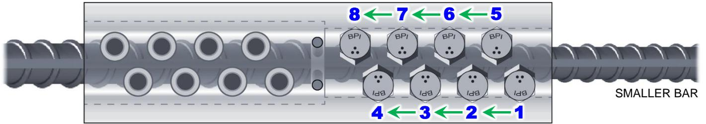
FIGURE 4. **Correct** Tightening Order, 2<sup>nd</sup> Side (#14 Transitions shown, #18 similar)
