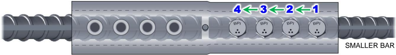
FIGURE 4: **Correct** Tightening Order, 2<sup>ND</sup> Side (#7/6 shown, other sizes similar)
