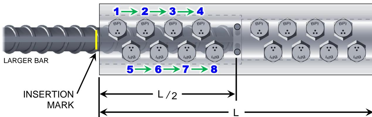
FIGURE 3: **Correct** Tightening Order, 1<sup>ST</sup> Side (#14 Transitions shown, #18 similar)
