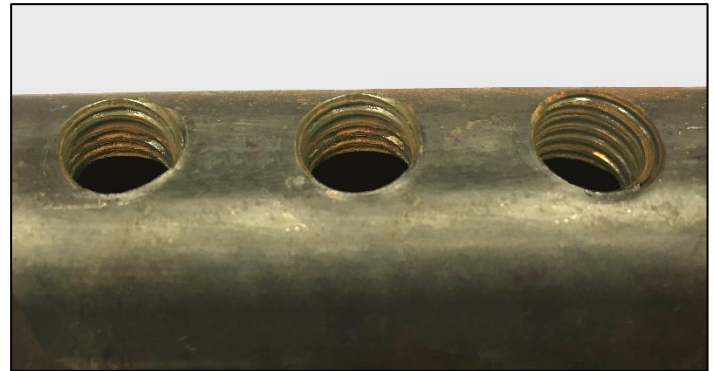
FIGURE 6: Unacceptable Rust in Connector Threads
