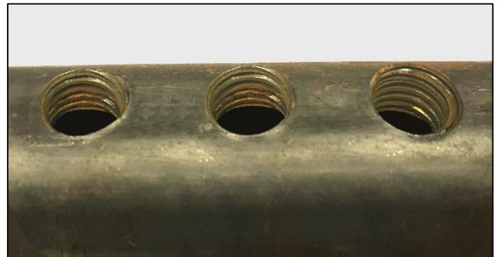
FIGURE 8: **Unacceptable** Rust in Threads
