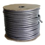
BoMetals Standard Backer Rod (FBR) is a ideal non aborbent compressible polyethylene material inserted into a joint to control sealant depth, creating a backstop to allow proper sealant tooling. It can also be used as a temporary joint seal.
