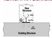
Used to provide a watertight seal when attaching a new construction project to an existing one.
